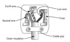
The wire coloured **BROWN** is the **LIVE** wire and must be connected to the terminal marked L or coloured **RED**.
