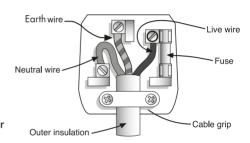
The wire coloured **BROWN** is the **LIVE** wire and must be connected to the terminal marked L or coloured **RED**.
